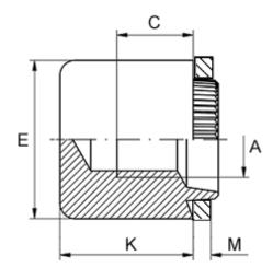
Female thread A = M10Height K = 14.0Min thread length C = 6.0Outer diameter E = 19.0Plate thickness = 2.0 to 2.2
